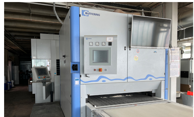
Pos. 124 1 Breitbandscheifmaschine BÜTFERING / WEEKE Profi SWT 335/HBB 1 Wide belt grinding machine BÜTFERING / WEEKE Profi SWT 335/HBB, YOM 2013
