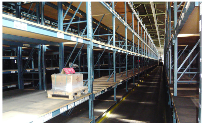
Pos. 439 686 lfm. Schwerlastregal (305 Elemente), B/T/H 2.000 x 850 x 5.000 mm 686 m. of Heavy-duty shelving (305 Elements), W/D/H 2,000 x 850 x 5,000 mm
