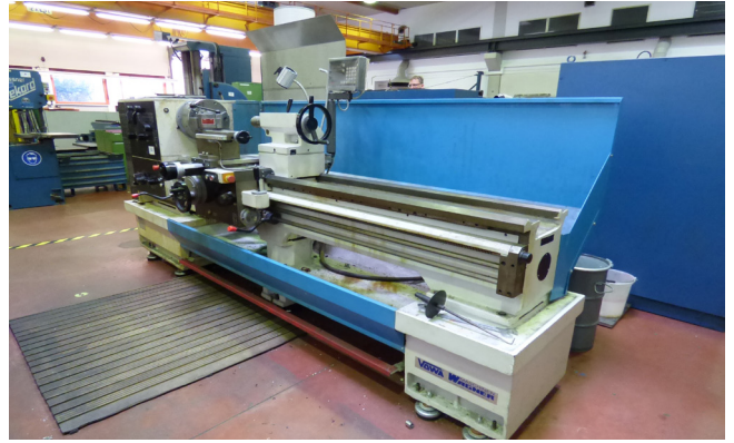
Pos. 12 1 L&Z Spindeldrehmaschine Chin. FABR. DCD330C x 2000, Bj. 2007 1 L&Z spindle lathe Chinese.built. DCD330C x 2000, YOM 2007
