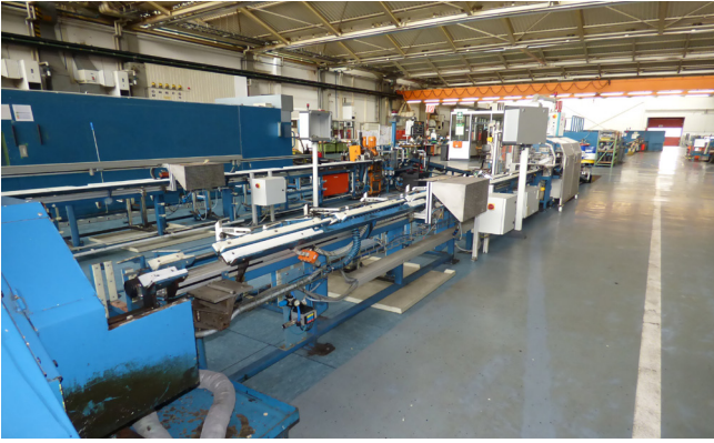
Pos. 161 1 Kaltpilgerwalzwerk KPW 222 SMS MEER, Bj. 1992 1 Cold pilger mill KPW 222 SMS MEER, YOM 1992
