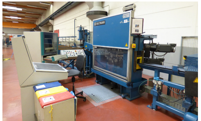
Pos. 264 16-Walzen-Richtmaschine BÜLTMANN DRM-R-60/HE, Bj. 1999 1 6-Roller levelling machine BÜLTMANN DRM-R-60/HE, YOM 1999
