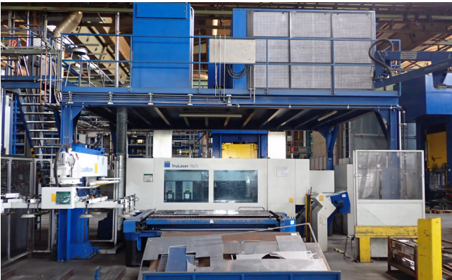
Pos. 378 1 CNC-Laserschneidanlage TRUMPF TRULASER 7025, Bj. 2007 1 CNC laser cutting system TRUMPF TRULASER 7025, YOM 2007
