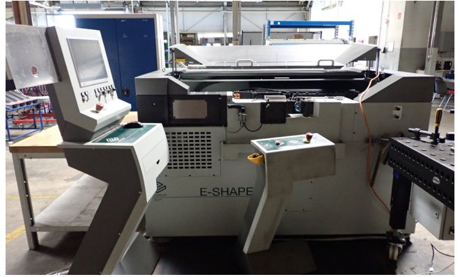
Pos. 692 1 Vollelekt. Rohrumformmaschine BLM E-SHAPE, Bj. 2017 1 Fully electr. tube forming machine BLM E-SHAPE, YOM 2017
