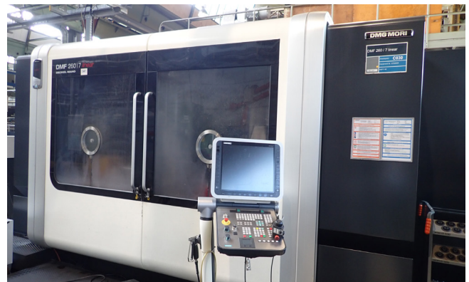
Pos. 347 1 CNC-Fahrständer-Fräsmaschine DECKEL MAHO DMF 260/7 LINEAR 1 CNC traveling column milling machine DECKEL MAHO DMF 260/7 LINEAR
