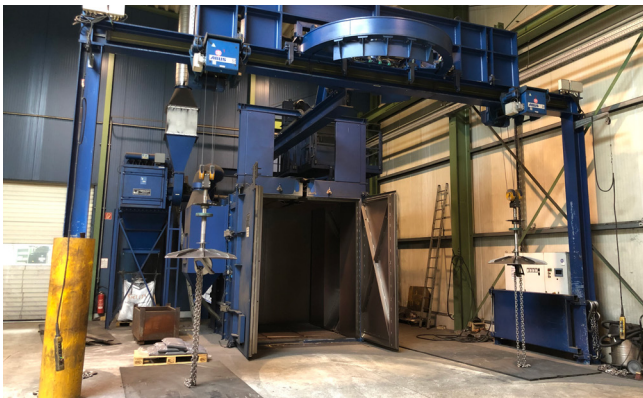
Pos. 3 1 Hängebahn-Strahlanlage RUMP 13E/VII, Bj. 2008 1 Overhead conveyor blasting machine RUMP 13E/VII, YOM 2008
