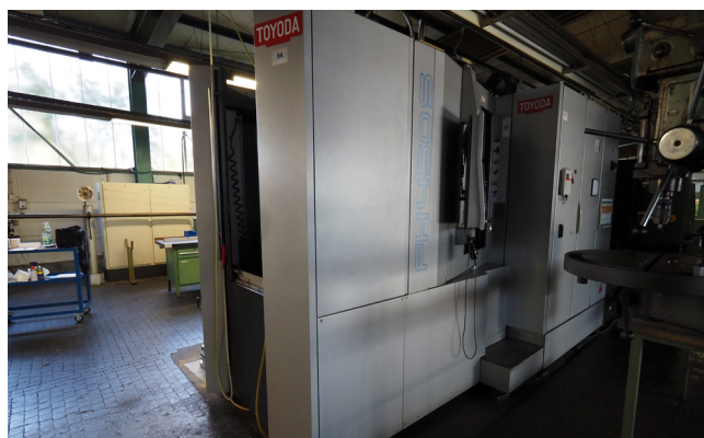
Pos. 94 1 horizontales Bearbeitungszentrum TOYODA FH 450S, Bj. 2007 1 Horizontal machining center TOYODA FH 450S, YOM 2007
