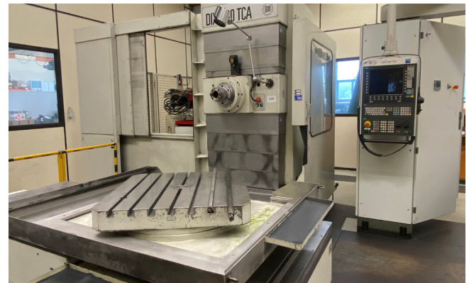
Pos. 110 1 CNC-Lehrenbohrwerk DIXI 280TCA 50S, Bj. 1990/2017 1 CNC Jig boring machine DIXI 280TCA 50S, YOM 1990/2017
