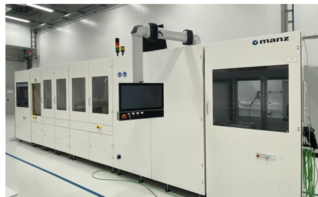
Pos. 6 1 Flexibles Laserschweißsystem MANZ BLS 500 (Battery Laser System) 1 Flexible laser welding system MANZ BLS 500 (Battery Laser System), YOM 2022
