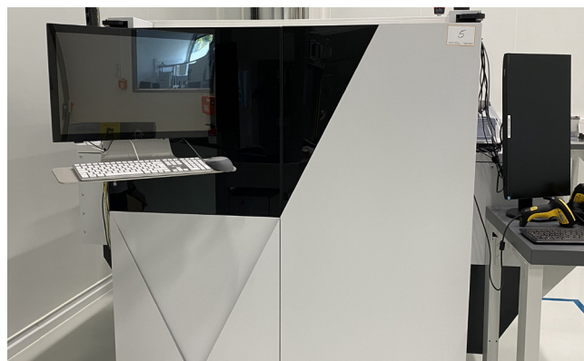
Pos. 5 1 Inline-Computertomograph Röntgenanlage ICT VISCOM IXCELL 1 Inline CT scanner X-ray system VISCOM IXCELL, YOM 2023
