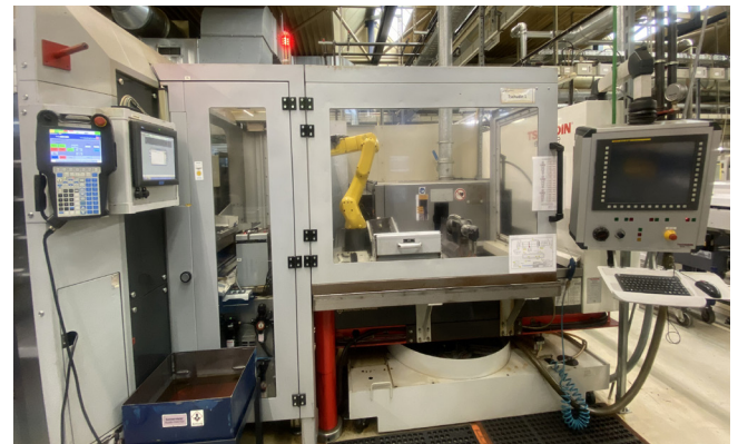
Pos. 16 1 CNC-Spitzenlosschleifmaschine TSCHUDIN ecoLine 400 CNC, Bj. 2015 1 CNC Centerless Grinding Machine TSCHUDIN ecoLine 400 CNC, YOM 2015
