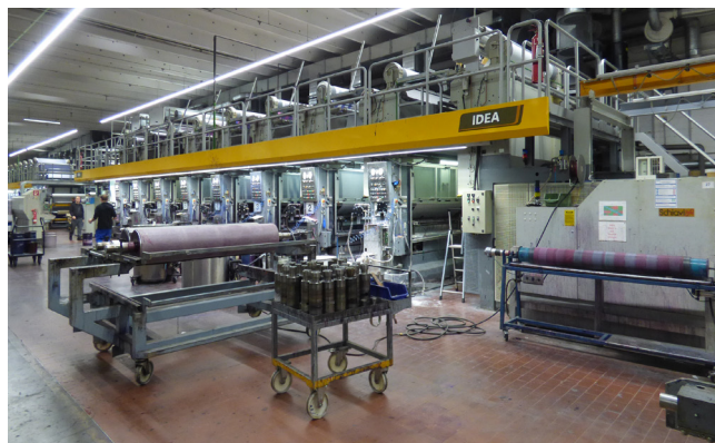
Pos. 27 18-Farben-Tiefdruckmaschine SCHIAVI Idea, Bj. 2002 18-Color gravure printing machine SCHIAVI Idea, YOM 2002
