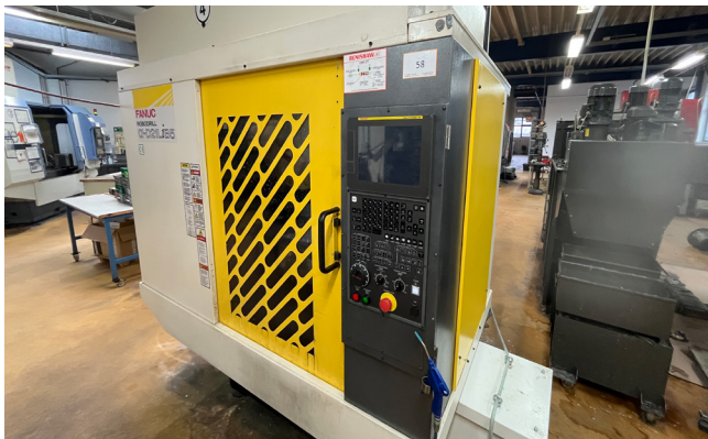
Pos. 58 1 Vert. Bearbeitungszentrum FANUC ROBODRILL Alpha-D21LiB5, Bj. 2018 1 Vertical machining center FANUC ROBODRILL Alpha-D21LiB5, YOM 2018
