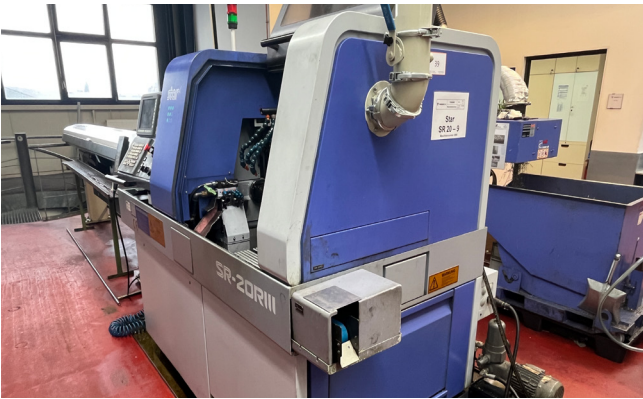
Pos. 39 1 CNC-Langdrehaautomat STAR SR-20 R III 680, Bj. 2011 1 CNC Swiss-type lathe STAR SR-20 R III 680, YOM 2011
