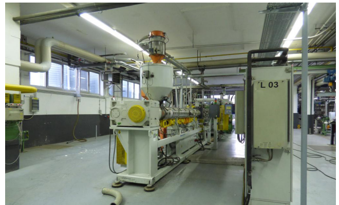
Pos. 3 1 Inline-Anlage „L03“ (Extruder & Thermoform-Maschine) BATTENFELD 1 Inline system "L03" (extruder and thermoforming machine BATTENFELD)
